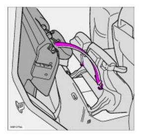
**NOTE:** Make sure that the holes in the plastic ferrules on the top of the backrest engage the hooks on the bottom of the seat cushion. When you later raise the backrest and seat cushion, the head restraints must be returned to their normal positions.
